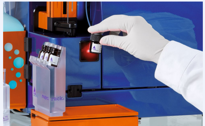
Figure 3: Reagent scanning for easy autolabeling.
